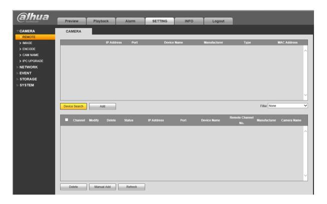
5. Go to "CAMERA → REMOTE". Click on "Device Search" to retrieve a list of cameras. Search for the one with the IP address of your DoorBird IP Video Door Station, mark its check box and click on "Add".
