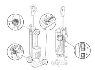
Unplug the vacuum before checking for blockages.
