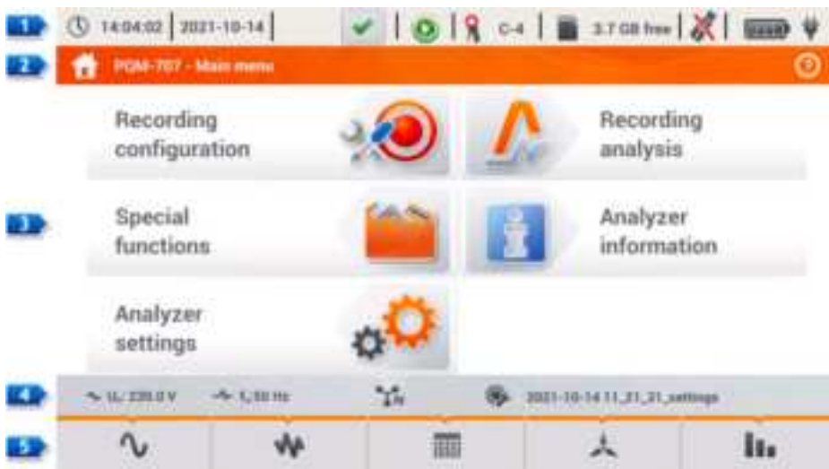
Fig. 2. Main elements of the analyzer screen.
