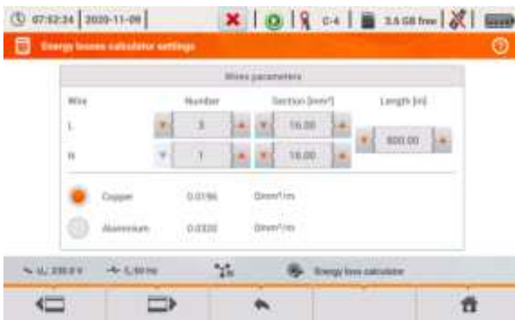
Fig. 50. Energy loss analysis – configuration screen 1
