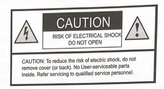
WARNING - To reduce the risk of electrical shock, do not remove cover (or open unit). NO USER SERVICEABLE parts are inside. Refer servicing to QUALIFIED SERVICE PERSONNEL.
