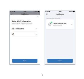
5. Manual configuration, when blue light of device blinks quickly, press Reset key for 5 seconds till the blue light blinks slowly, click "+" in top of right or "Add device" in middle blank by APP home page, choose "sensors"  $\rightarrow$  "CO alarm(WiFi) $\rightarrow$ indicator light blinking slowly → input WiFi password(support 2.4G WiFi only, not 5G) → choose "Smartlife\_XXXX" from WiFi list → return to App and manual configuration success.
