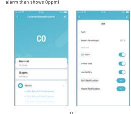
7. It reports to APP automatically when there is malfunction with CO sensor, the orange indicator light flashes twice every 40 seconds, the buzzer beeps twice, and the screen shows "ERR."
