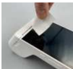
5. Remove the excessive paper by tearing along the serrated edge.
