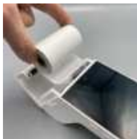
2. Insert the paper roll in the compartment following the directions shown in the picture.
