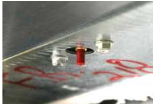
The hi-limit reset is accessible in the fryer cabinet under the controller.
