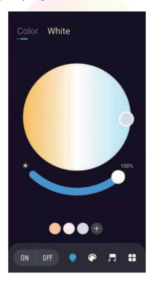
7.Click the color light in the upper left corner to switch to the color light adjustment page. The color of the color light can be adjusted in the circular area above, and the brightness of the arc-shaped adjustment rod below can be 1% - 100%.
