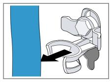
2. Unscrew 1 and remove 2 all of the screws for the 4 transit bolts using a WAF 13 wrench.
