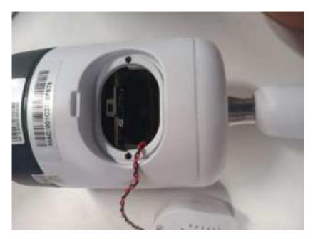
Step 2. Insert the micro Micro SD card just like the way in the picture below, please use your fingernail (or use the provided reset needle) to push the micro Micro SD card in until it is locked, and you will hear a click sound and the micro Micro SD card will not pop out if it is inserted in properly.
