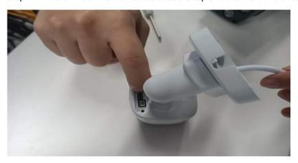
Step 2. Insert the micro Micro SD card just like the way in the picture below, please use your fingernail (or use the provided reset needle) to push the micro Micro SD card in until it is locked, and you will hear a click sound and the micro Micro SD card will not pop out if it is inserted in properly.
