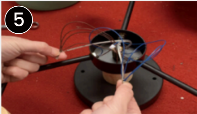
Twist the wires of the same color together, and give the white wires to the red and blue wires respectively
