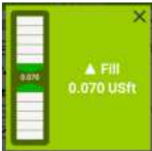
Fill, within Surface Stakeout Tolerance
