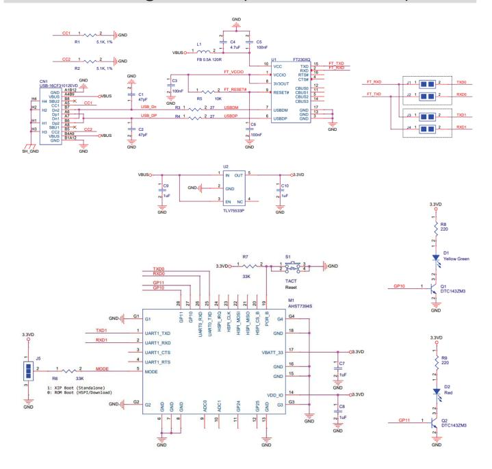
HSPI and UART1 are the general interfaces used for external host MCU. The HSPI is a specially designed SPI for high-speed data transfer.
