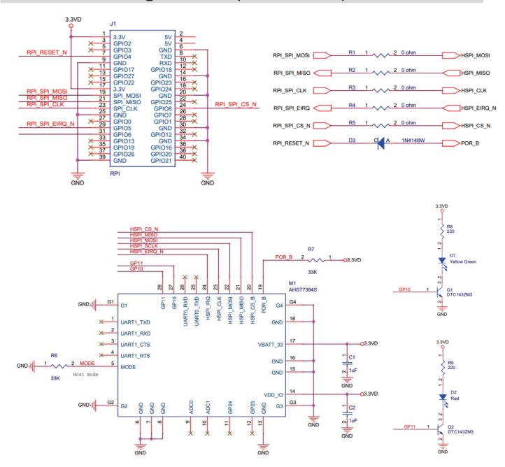
HSPI and UART1 are the general interfaces used for external host MCU. The HSPI is a specially designed SPI for high-speed data transfer.
