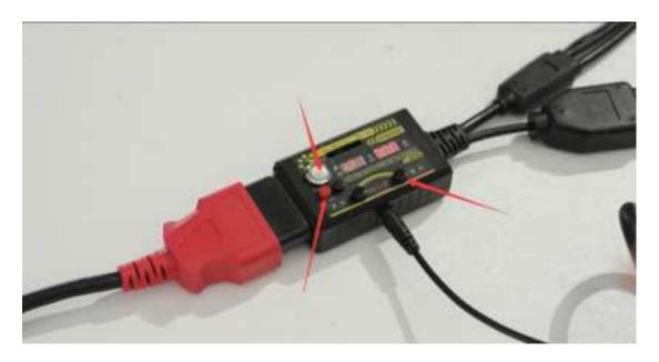
Step 3: Press in sequence: power switch start, ignition switch IGN, engine button switch ENG.
