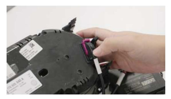
Step 3: Connect the instrument.
