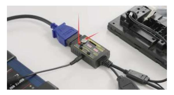
Step 6: Press the start button and the red ignition switch button again.
