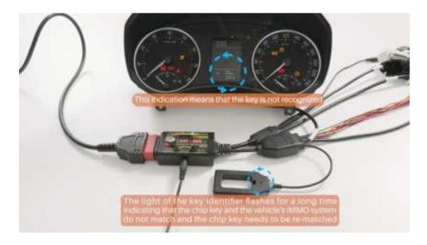
Step 1: Connect the GT115 to the dashboard and connect it to the power supply.
