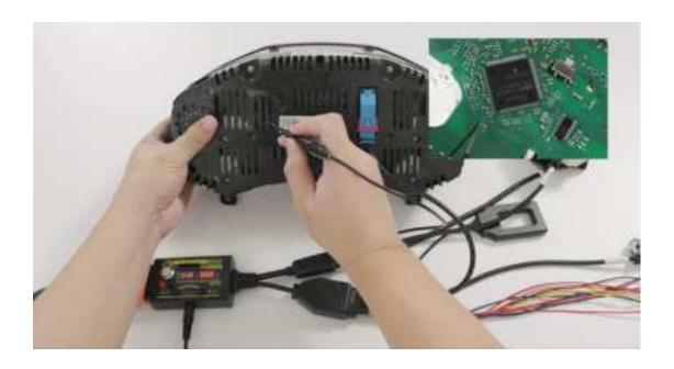
Step 3: Then use the pogo pin probe to poke the pogo pin point in the instrument chip.
