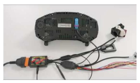
Step 1: Connect GT115 to the instrument panel and power it on.
