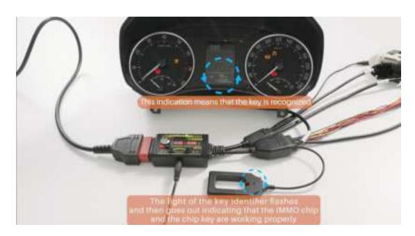
Step 4: Connect the GT115 to the dashboard and connect it to the power supply.
