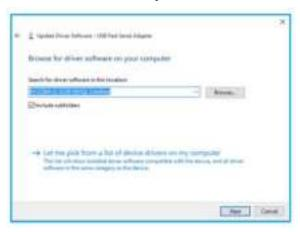
In the address box, put the exact location where the Windows drivers have been saved to. After entering the address select "Next" to start the installation.
