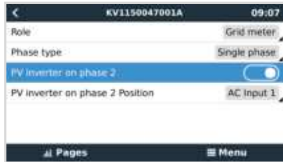
Single-phase, dual function to measure grid on L1 and a PV Inverter on L2
