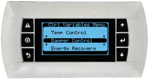
Figure 17: Ctrl Variables Menu shown on a handheld keypad/display
