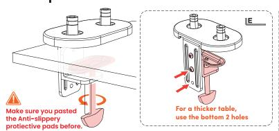
Clamp the base on the table and fix it in place.
