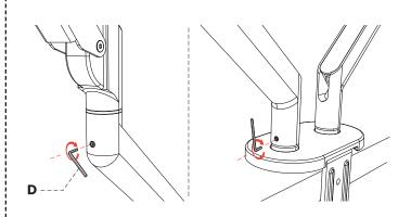
Tighten the screw to lock the rotation if needed.
