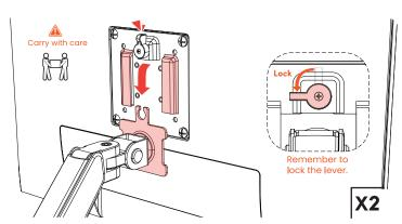
Attach the monitor to the arm and turn the lock.
