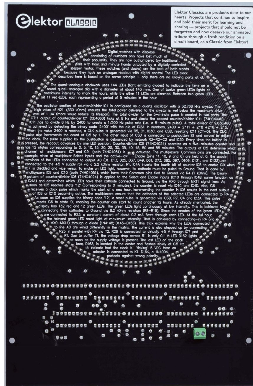
Figure 5: View of back of PCB 240118-1 v1.1. All parts are fitted and soldered.
