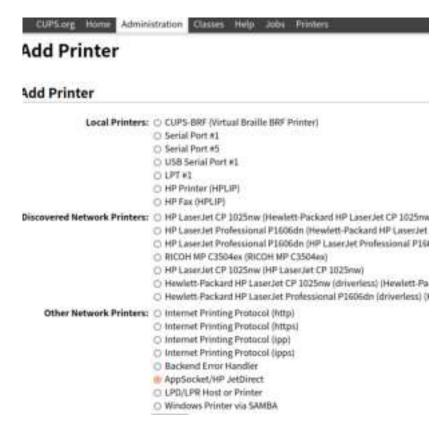
5. Enter the printer's IP address, e.g. socket://10.3.9.55:9100.
