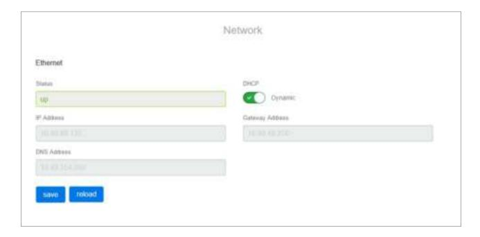
4. If charger has a hardwired connection but Ethernet status is Down & Red call EO for further support.
