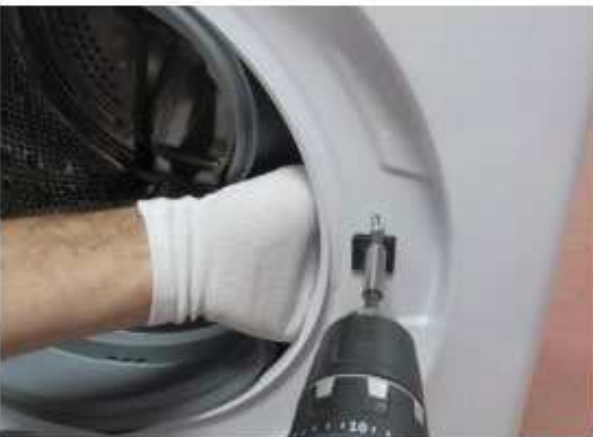
Tighten the door lock screw
