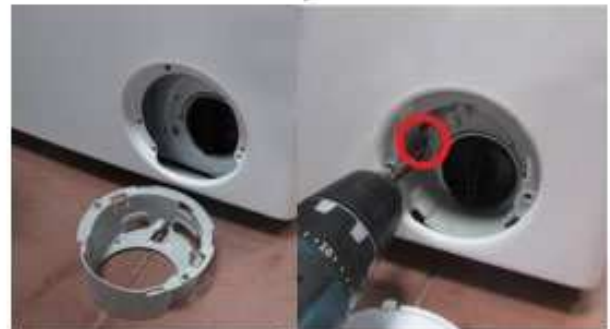
Tighten the screw fixing the front panel at the bottom
