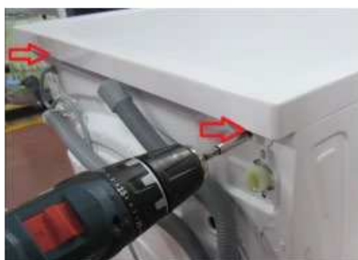
Remove two screws that fix the top-plate at the back.
