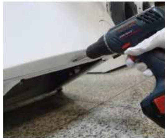
Tighten the screw fixing the front panel at the bottom
