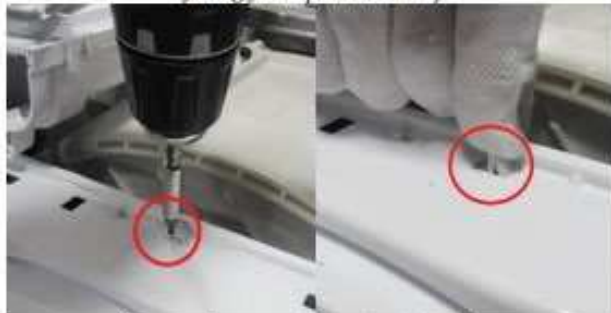
Remove the screw fixing twinjet elbow.
