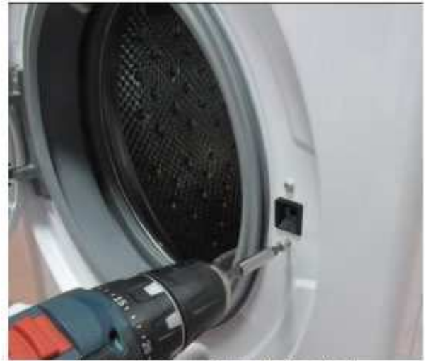
Remove the screws fixing the door lock.
