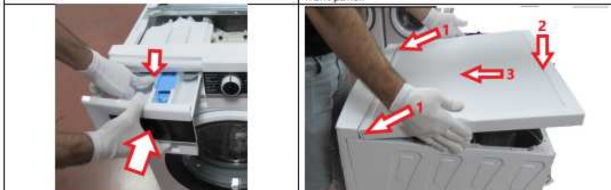
3.12. While pressing siphon cover keep pushing
