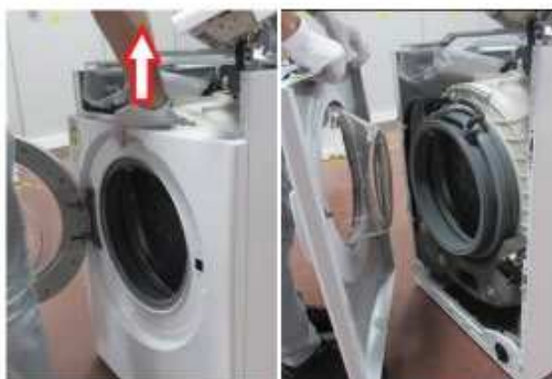
Pull up and remove the front panel.
