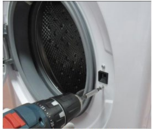
Remove the screws fixing the door lock.
