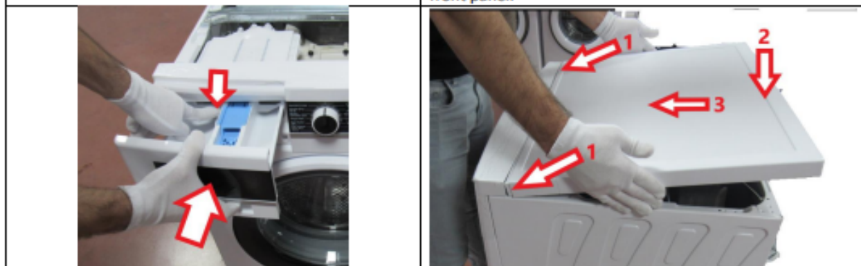
3.12. While pressing siphon cover keep pushing
