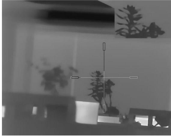
Figure 6-1 PIP Effect in Correcting Reticle
