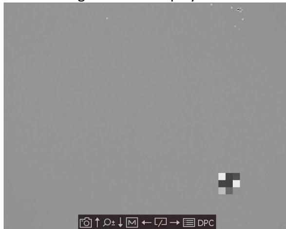
Figure 3-3 Correct Defective Pixel
