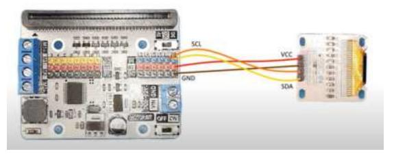
Make sure the Slide switch is set to 3V3
