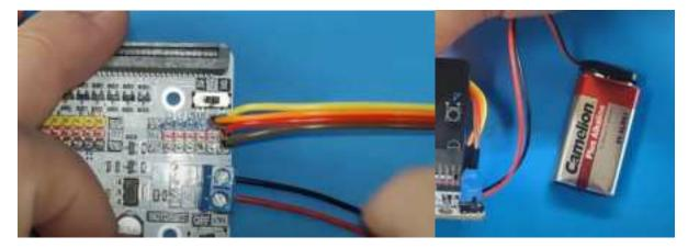
Connect the Micro Bit and set the ON/OFF switch of the motor board to ON.
