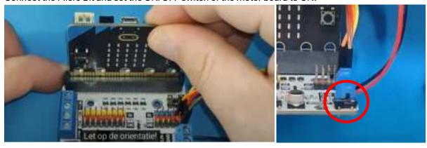
Press the RESET button on the back of the Micro Bit, and the OLED screen should light up. Now follow the instructions on the screen.
