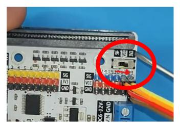
Now connect the battery using the 9V battery clip and connect the wires to the terminal on the Motor Shield, Dont switch the wires!
