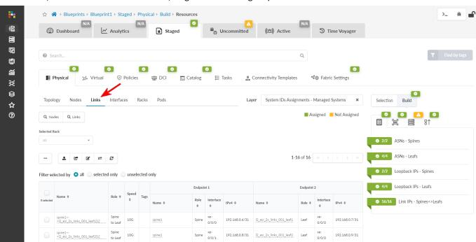
2. Review the calculated cabling map and cable up the physical devices according to the map. If you have a set of precabled switches, ensure that you have configured interface maps according to the actual cabling so that calculated cabling matches the actual cabling.
