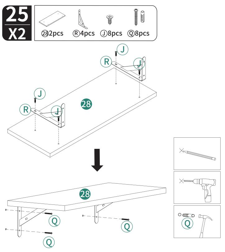
Note: Before drilling holes to the wall, please confirm the position first and mark the drilling locations with a pen. (The above picture is just for reference)
