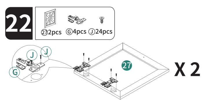
In order to ensure the consistent spacing between the upper and lower door joints, the lower part of the door hinge should be installed first, followed by the upper part.
