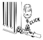
5 Repeat step 3 and 4 until all valves have been set correctly. Sensor may now be fitted or the valve cap temporarily refitted.
