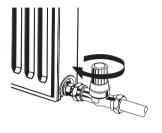
Close all radiator valves by turning the valve cover cap clockwise. Leave system to cool.
