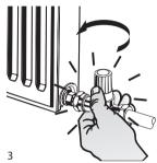
Open one valve and determine flow direction. Which pipe heats first?
