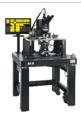
Example configuration pictured above: M-8 manual probe station with a vibration isolation table incorporating a rapid advance wafer stage, 200 mm tilting chuck, platen with linear lift, DC manipulators, compound optics and CCTV system.
