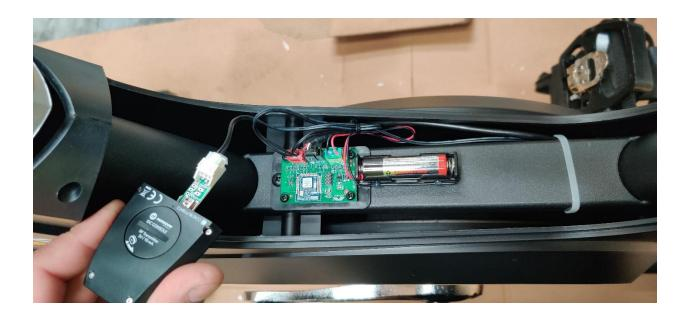
**Step 5.**Mount the sender on to the frame, under the seat.
