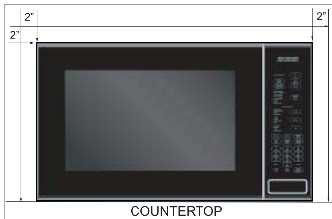
Figure 2-2. 2" Clearance on Sides, Top & at Rear
