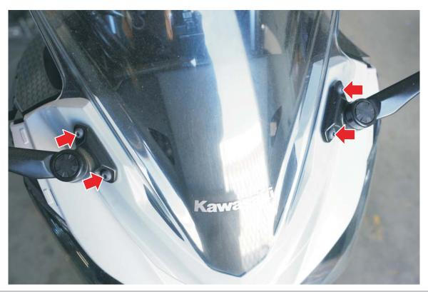
7. Remove nose fairing/headlamp assembly. Cut both the cables ties securing the low and high beam /DRL harness to the head light sub-frame. Remove 2 bolts on each side using 10mm socket, 1 on the upper side and 1 on the lower bottom.
