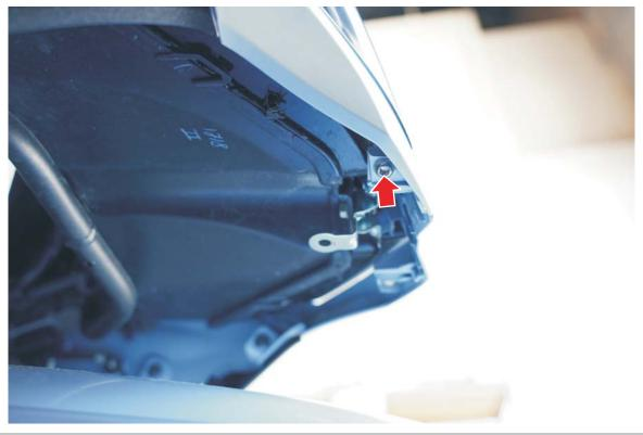
Step 5 continued - 1 bolt at the rearmost fairing using 5mm allen tool
