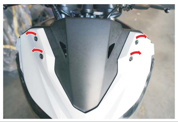
9. Reach in and undo the 2 wire management clips, slide off the boots and unplug the low beam, high beam, and 2 DRL connector plugs. At this time, the entire nose fairing/head light assembly can be removed
