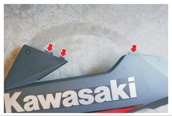
2. Remove center wheel well panel. 3 plastic fasteners per side, 1 plastic fastener at the upper middle and 1 bolt on each side using a 10mm socket. Release the several tabs on each side and pull forward to remove
