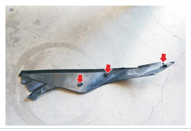
5. Remove upper side fairing assembly. 1 bolt right up front below head light using 4mm allen. 1 bolt at the rearmost fairing 5mm allen, this bolt has a shouldered washer. 1 bolt at the lower (8mm socket) and uppermost (10mm socket) of the fairing. Support fairing on the last bolt. Carefully remove the fairing, un-clipping the 4 locking tabs and 1 plastic fastener in the area below the handle bar. Unplug turn signal. Repeat other side.
