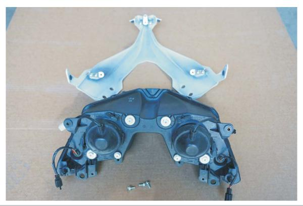
11. Swap over both the metal collars and rubber grommets at the lower mount to the new LED head light. The collars insert from front to back.
