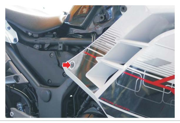
Step 5 continued - 2 bolts: upper using 10mm socket and lower using 8mm socket
