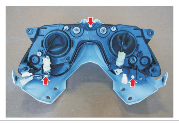
14. Mounting the head light/nose fairing assembly back onto the bike. While keeping the towel on the front fender, carefully position and rest the assembly on the towel then plug in the low beam, high beam, left DRL and right DRL plugs, cover with rubber boot.
