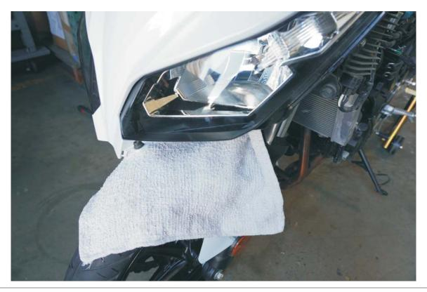
Step 8 continued - lift up and out at the mirror standoffs to release the fairing/head light assembly and carefully place on top of towel.
