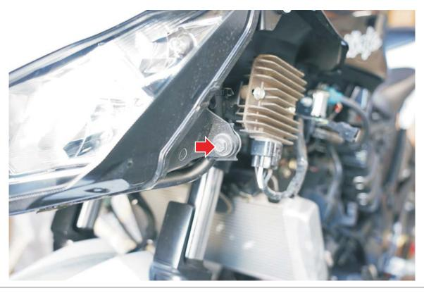
Step 7 continued - 1 bolt lower right using 10mm socket
