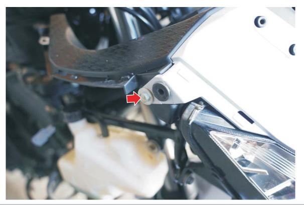
Step 7 continued - 1 bolt lower left using 10mm socket
