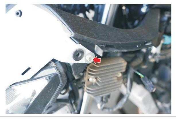
Step 7 continued - 1 bolt upper right using 10mm socket
