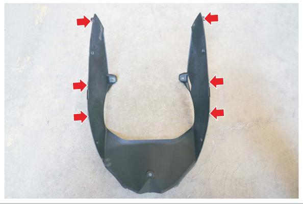
3. Remove painted side panel. 1 bolt using 4mm allen and pull towards you to remove, it is held on by 4 friction fasteners. Repeat other side
