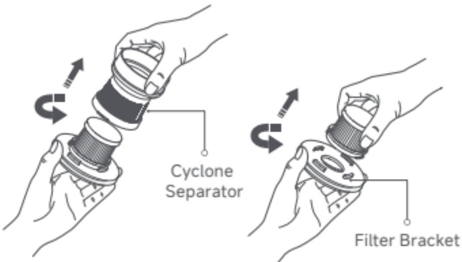
3. Turn the new filter clockwise onto the filter bracket to install it.
