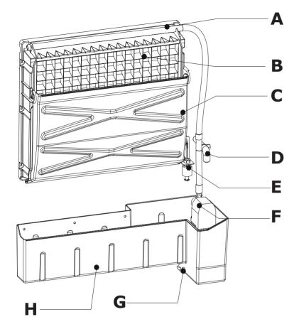
**A.Water dividing pipe**: With seventeen little holes, water will flow out from these little holes. And if no water flows out, it can be disassembled and cleaned
