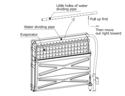
3. When there are ice cubes on the surface of the evaporator, but they can't fall down easily, do not use the mechanical substance to remove the ice cubes by force; Only press the "ON/OFF" button for more than 5 seconds, the unit will enter the ice melting process, after a while, the big ice cubes will fall down, then turn off the unit and unplug the power cord to clean the surface of the evaporator.
