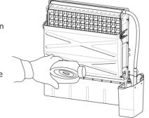
7.Turn on the power to the ice maker, then press "TIMER CLEAN" button on control panel for more than 5 seconds, to enter the self-Cleaning program. The machine will start self-cleaning when the water is enough, The symbol will revolve on The LCD , display The "90" countdown time. Stop working after 90 minutes.
