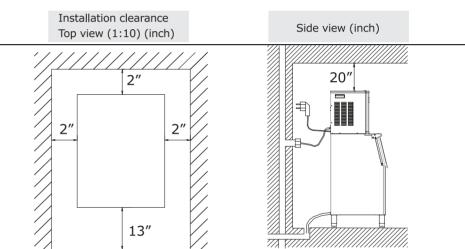
To ensure proper ventilation for your ice maker, the top of the unit must be completely unobstructed (at least 20 inch free space). Allow at least 2 inch clearance at rear, and 2 inch at sides for proper air circulation. The installation should allow the ice maker to be pulled forward for servicing if necessary.
