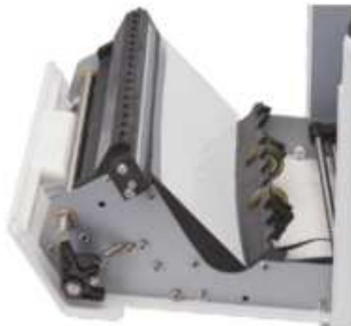
Figure 7 - 21 Place the CIS Calibration Paper
