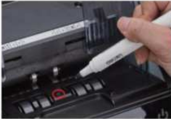
Figure 7 - 27 Use Marker Pen to Decrease the Sensitivity of Hopper Sensor
