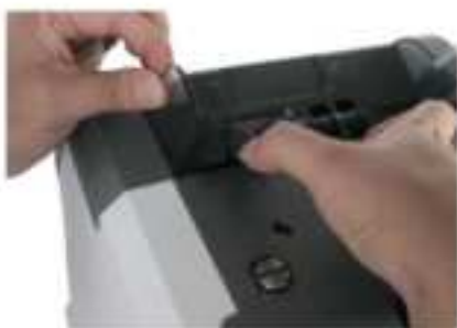
Figure 2 - 3 Banknote Guider Uninstallation
