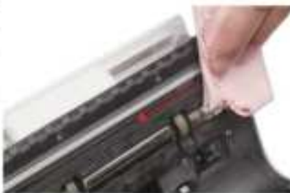
Figure 7 - 8 Clean the Lower CIS
