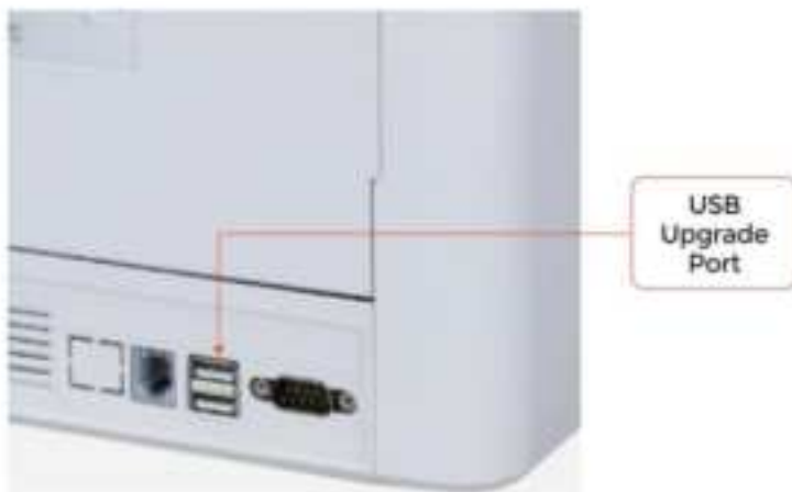
Figure 6 - 1 USB Upgrade Port
