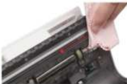
Figure 7 - 8 Clean the Lower CIS
