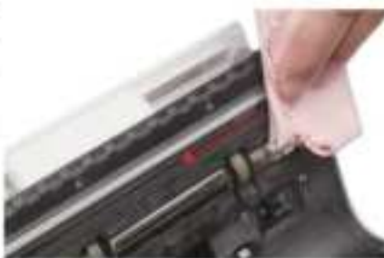
Figure 7 - 8 Clean the Lower CIS
