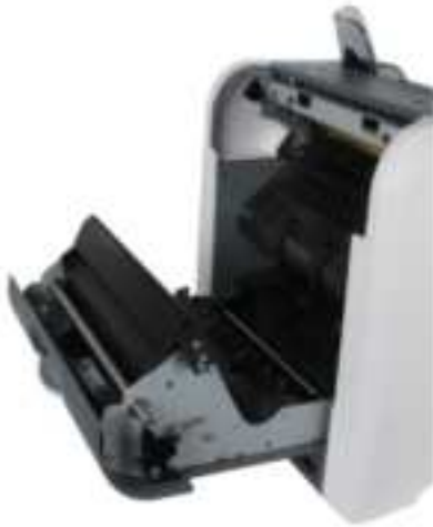
Figure 7 - 19 Open the Back Covers
