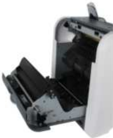
Figure 7 - 19 Open the Back Covers
