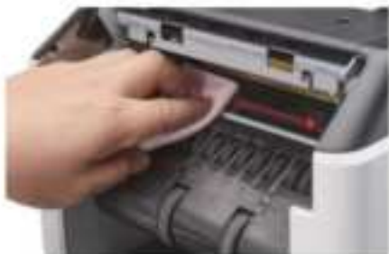
Figure 7 - 7 Clean the Upper CIS
