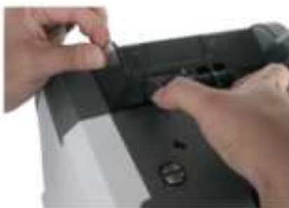
Figure 2 - 3 Banknote Guide Uninstallation
