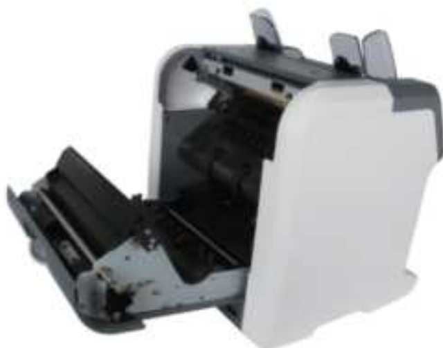
Figure 7 - 3 Handle of Back Cover
