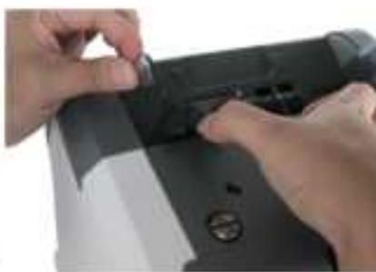
Figure 2 - 3 Banknote Guider Uninstallation
