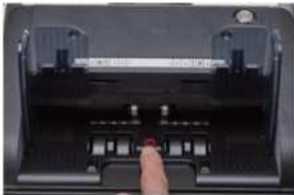
Figure 7 - 26 Touch the Hopper Sensor
