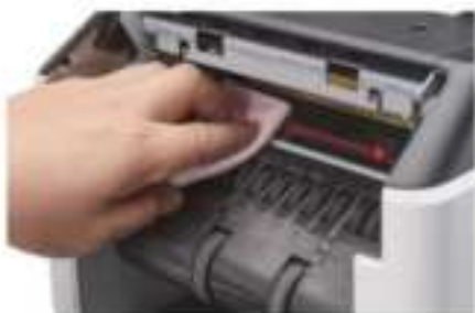
Figure 7 - 7 Clean the Upper CIS
