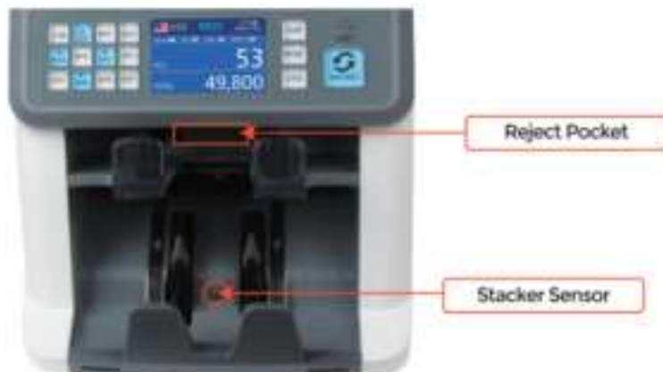
Figure 7 - 2 The Sensors in Stacker and Reject Pocket
