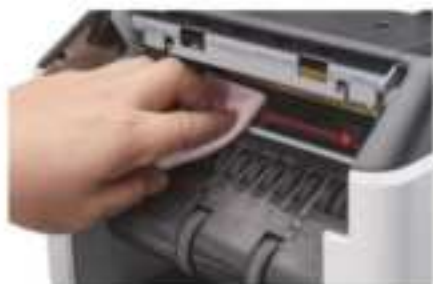
Figure 7 - 7 Clean the Upper CIS
