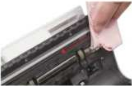
Figure 7 - 8 Clean the Lower CIS
