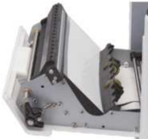
Figure 7 - 21 Place the CIS Calibration Paper
