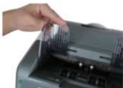
Figure 2 - 2 Banknote Guider Installation
