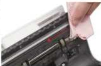
Figure 7 - 8 Clean the Lower CIS
