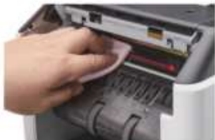
Figure 7 - 7 Clean the Upper CIS
