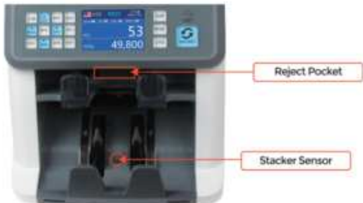
Figure 7 - 2 The Sensors in Stacker and Reject Pocket
