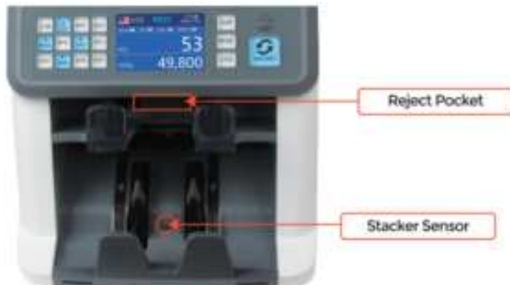
Figure 7 - 2 The Sensors in Stacker and Reject Pocket
