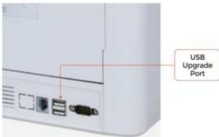
Figure 6 - 1 USB Upgrade Port
