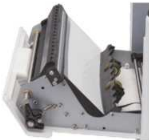
Figure 7 - 21 Place the CIS Calibration Paper
