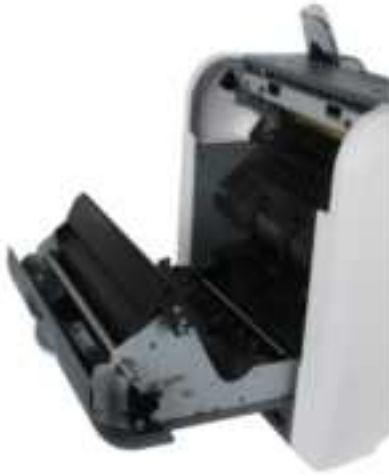
Figure 7 - 19 Open the Back Covers
