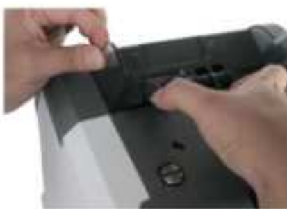
Figure 2 - 3 Banknote Guider Uninstallation
