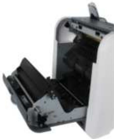
Figure 7 - 19 Open the Back Covers
