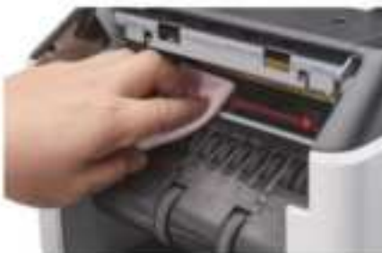
Figure 7 - 7 Clean the Upper CIS
