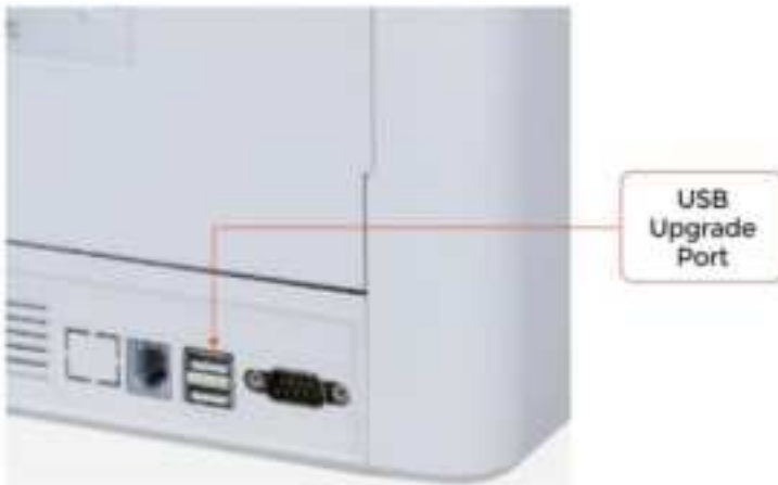
Figure 6 - 1 USB Upgrade Port
