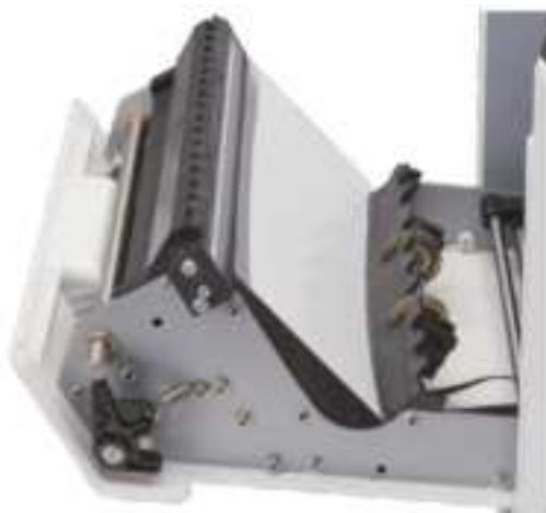
Figure 7 - 21 Place the CIS Calibration Paper
