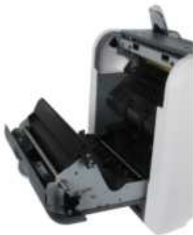
Figure 7 - 19 Open the Back Covers
