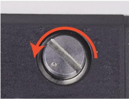
Figure 7 - 12 Rotate the Screw to Decrease the Feeding Gap
