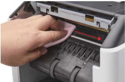
Figure 7 - 7 Clean the Upper CIS
