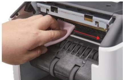
Figure 7 - 7 Clean the Upper CIS
