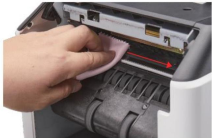
Figure 7 - 7 Clean the Upper CIS
