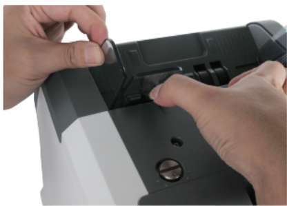
Figure 2 - 3 Banknote Guider Uninstallation
