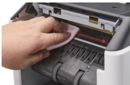
Figure 7 - 7 Clean the Upper CIS
