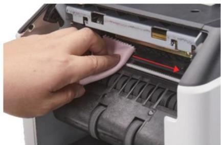
Figure 7 - 7 Clean the Upper CIS
