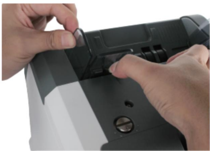
Figure 2 - 3 Banknote Guider Uninstallation
