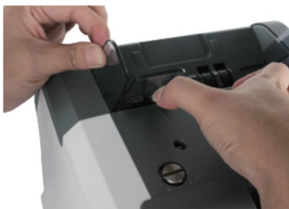
Figure 2 - 3 Banknote Guider Uninstallation
