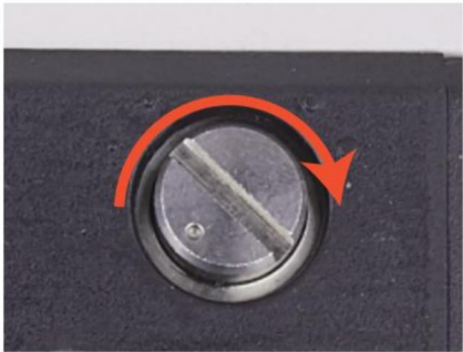
Figure 7 - 11 Rotate the Screw to Increase the Feeding Gap
