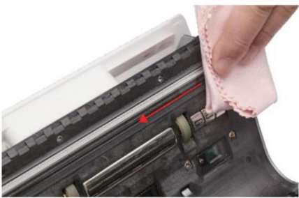
Figure 7 - 8 Clean the Lower CIS
