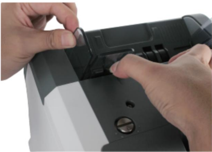
Figure 2 - 3 Banknote Guider Uninstallation
