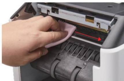
Figure 7 - 7 Clean the Upper CIS
