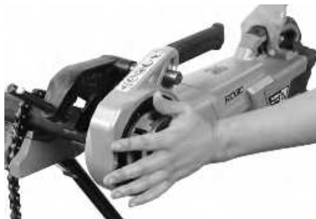
Figure 13A – Starting the Thread Using the Die Head Cover Plate
