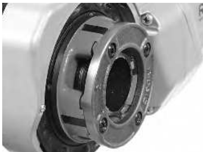
Figure 15 – Pipe Even with Edge of Dies
