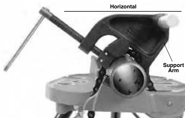
Figure 10A – Positioning the Support Arm
