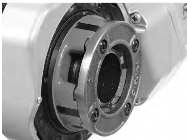
Figure 15 – Pipe Even with Edge of Dies
