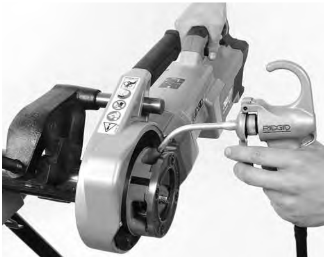
Figure 14 – Filetage du tuyau
