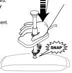
Pump is fully engaged when top surface of pouch fitment touches pump connector rim.
