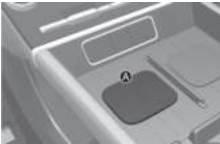
[A] Vehicle authentication pad (Wireless charging pad)
