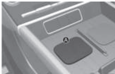
[A] Vehicle authentication pad (wireless charging pad)
