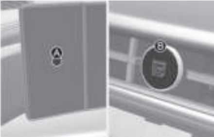
[A] Fingerprint sensor [B] Engine Start/Stop button
