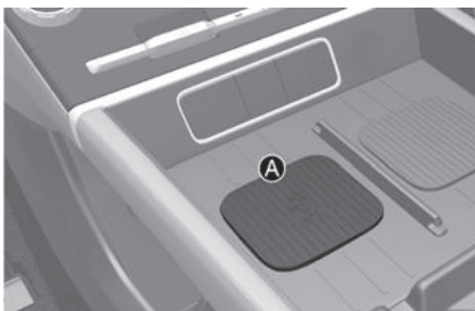
[A] Vehicle authentication pad (Wireless charging pad)
