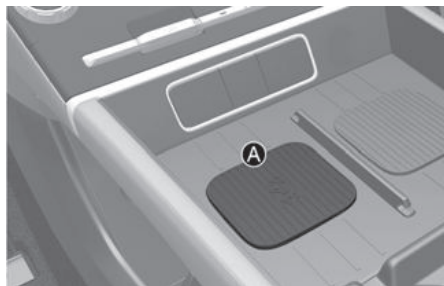
[A] Vehicle authentication pad (wireless charging pad)
