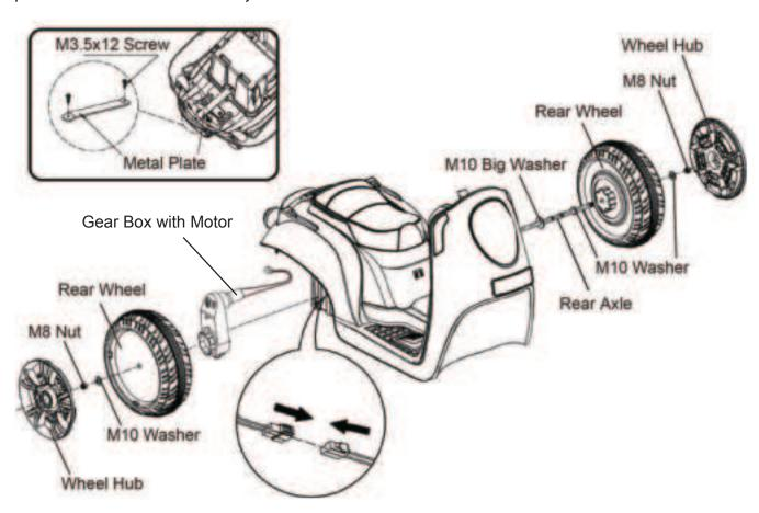
The M8 Nuts and Washers pre-installed on the rear axle, dis-assemble them except the Big washer (keep the big washer), then insert the rear axle through the vehicle body.
