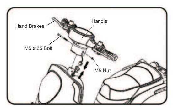
Assemble the handle on the front axle, then secure using a M5  $\times$  65 bolt and a M5 nut. **NOTE: Hand brakes have no actual function.**
