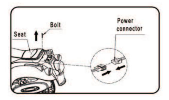
Remove the seat from the vehicle. The wire connector plug butt. Replace the seat and secure using the removed bolt.
