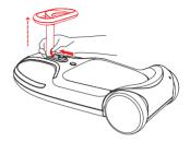
Uncover the hole for the support column at the front of the vehicle body, then insert the support column into it. Make sure that the groove is aligned with the limit position.
