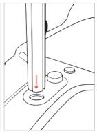
Insert the support column into the handlebar, aligning the groove with the limit position.
