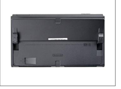
• Use a Y00 screwdriver to remove the two 4.3 mm screws securing the rear case to the frame.
