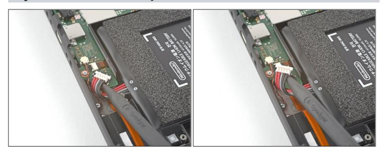
• Use the point of a spudger to pry up and disconnect the battery.
