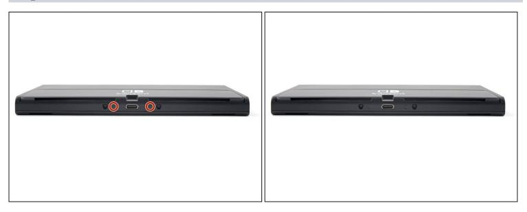
• Use a Phillips driver to remove the two 2 mm-long screws securing the bottom of the rear case to the frame.
