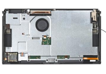
• Use a Phillips driver to remove the 4.4 mm screw securing the secondary Wi-Fi antenna to the shield plate.
