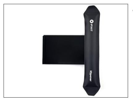
Apply a <u>heated iOpener</u> to the right edge of the screen for 90 seconds to loosen the adhesive underneath.
