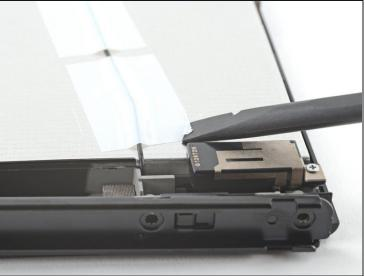
• Use the flat end of a spudger to separate a corner of the tape from the shield plate.
