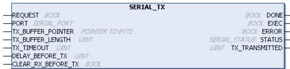
Figure 124: Block for Values Transmission by the Serial
