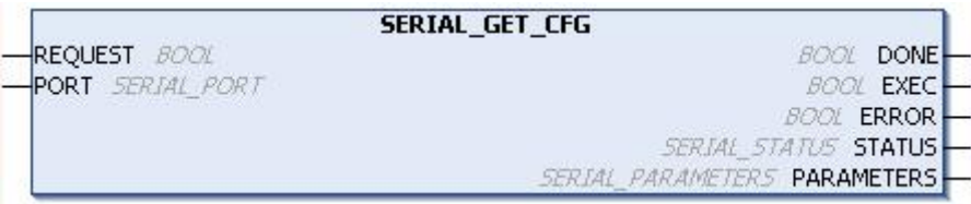
Figure 117: Block to Capture the Serial Configuration
