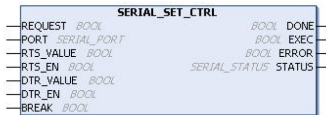
Figure 123: Block for Control Signals Writing
