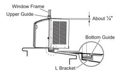
2 Extend the guide panels to fill the window opening and use 2 type B screws and 2 type C screws to secure them
