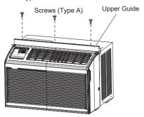
Insert the top and bottom rails of the curtain panels into the upper and lower panel guides Fasten the curtain panels to the unit with 8 type A screws Fasten screws behind the curtain panel.
