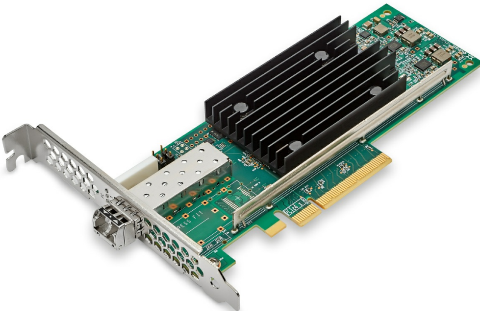
Figure 2. ThinkSystem QLogic QLE2770 32Gb 1-Port PCIe Fibre Channel Adapter
