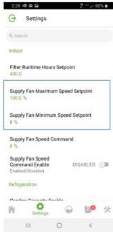
Figure 24. Supply Fan speed setpoints
